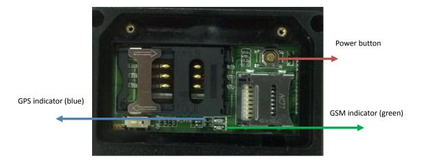
To start the device, press and hold down the power button for 3–5 seconds, or connect the device to external power supply.
