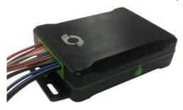
Note: The device side with the Meitrack logo faces upwards to get better GPS signal.
